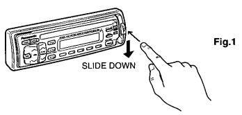
③ Remove the removable face plate by pulling on the right side of the unit. Place the removable face plate in a supplied case.
